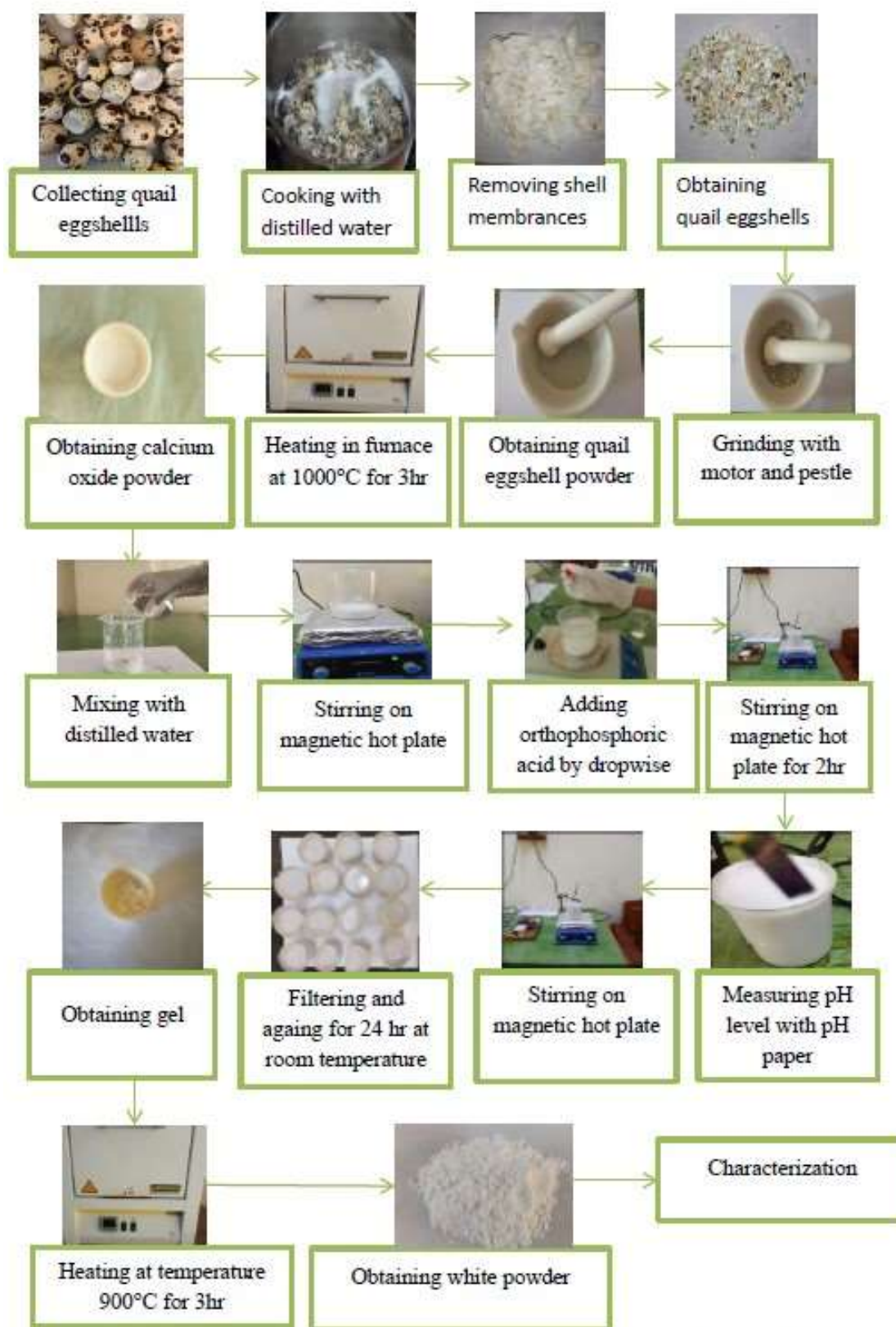
Figure 2. The sample preparation of hydroxyapatite powder from quail eggshells by precipitation method
