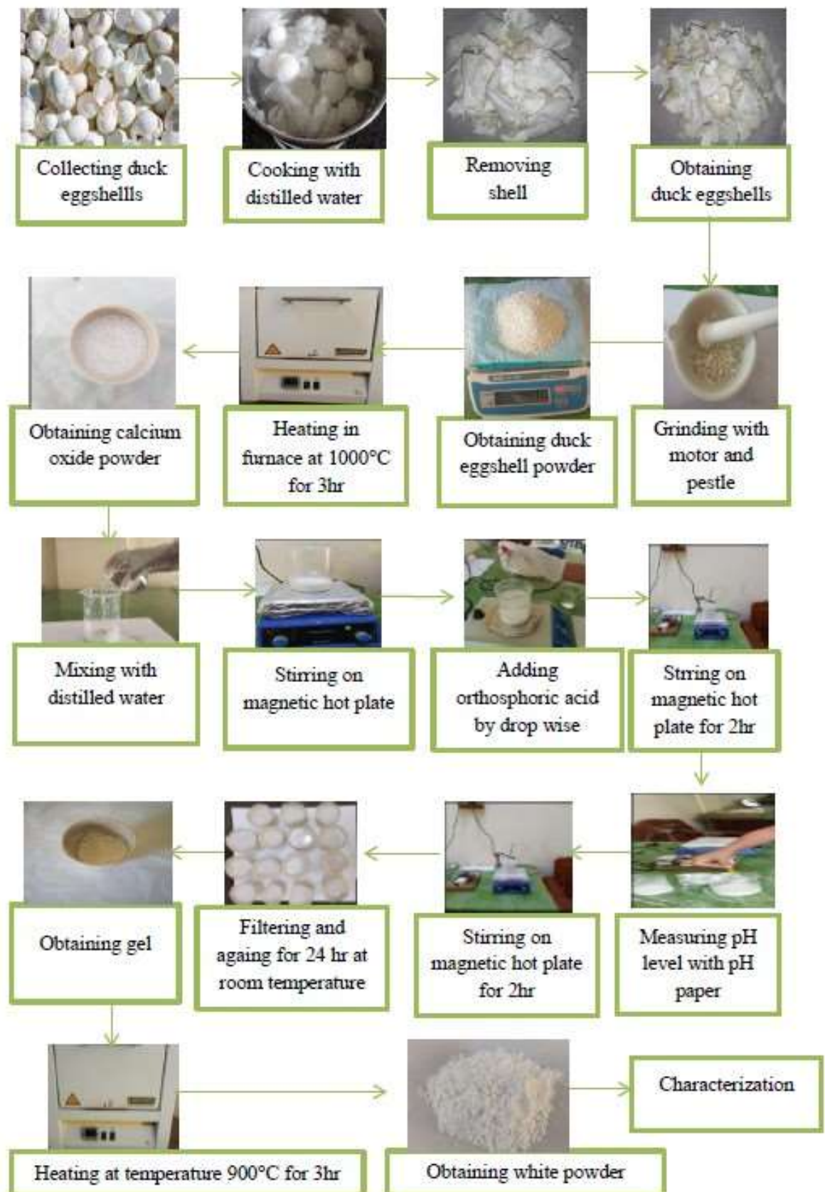
Figure 3. The sample preparation of hydroxyapatite powder from duck eggshells by precipitation method
